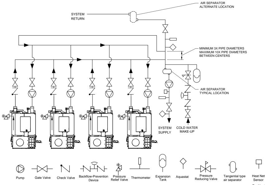
For Heat-Net operation, a sensor is required and installed at a minimum of 12" from primary loop tee.
